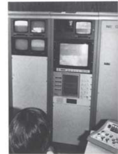
Fig. 2. Monitoring Station. The UI consultant, controlling the mobile camera at FCH remotely, views medical personnel and patients on a 19-inch color screen.
